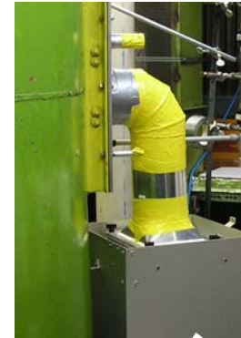
3. High Volume Filter Sampling of Primary Smoke PM 2.5 (quartz substrate)
