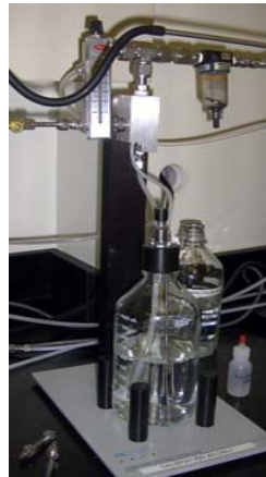
5. Aerosol Generation with Aqueous or Methanol Solution
